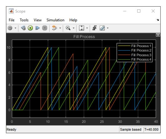
In the second scope, observe the number of trucks leaving after being filled. The plot displays that there are 15 trucks leaving the facility after their gas tanks were filled.
